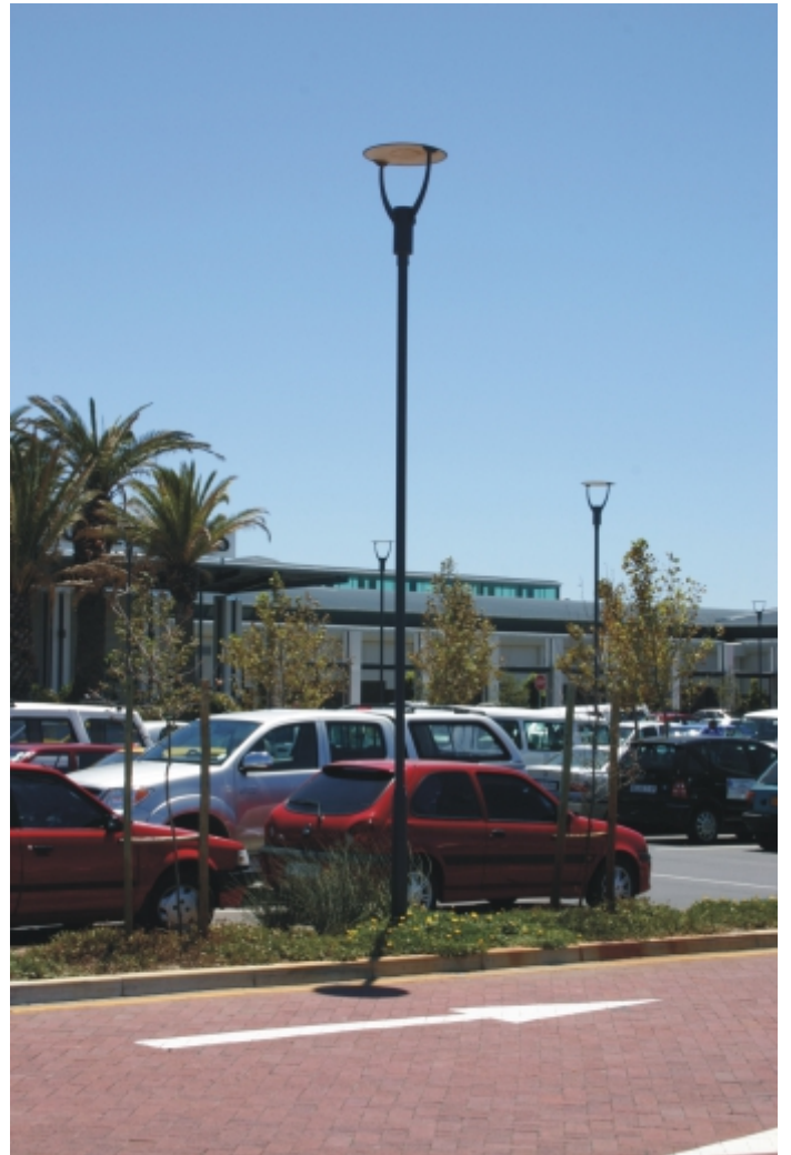
Saturn post top 150W MH on a 4m MH Pole
