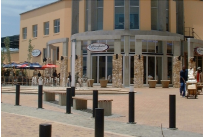
Shaft bollard with matching non illuminated bollard and Beam up down lighters on the pillars
